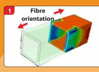
Finalisation of design is based on FE simulations of composite materials
